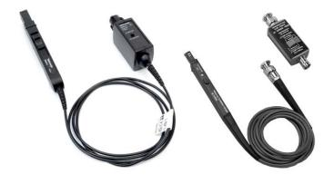
The P6021 and P6022 Current Probes provide versatile AC current measurements. Both probes provide accurate current measurements over a wide range of frequencies. The P6021 and P6022 allow current measurements without breaking the circuit by clipping onto the current carrying conductor. Shielded probe heads are not grounded when the slides are in their open positions, eliminating accidental grounding of the circuit under test.
